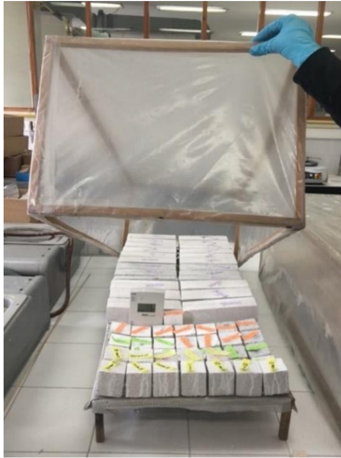
Figure 3.4. Carbonation process of AAC samples in a chamber with high relative humidity.
