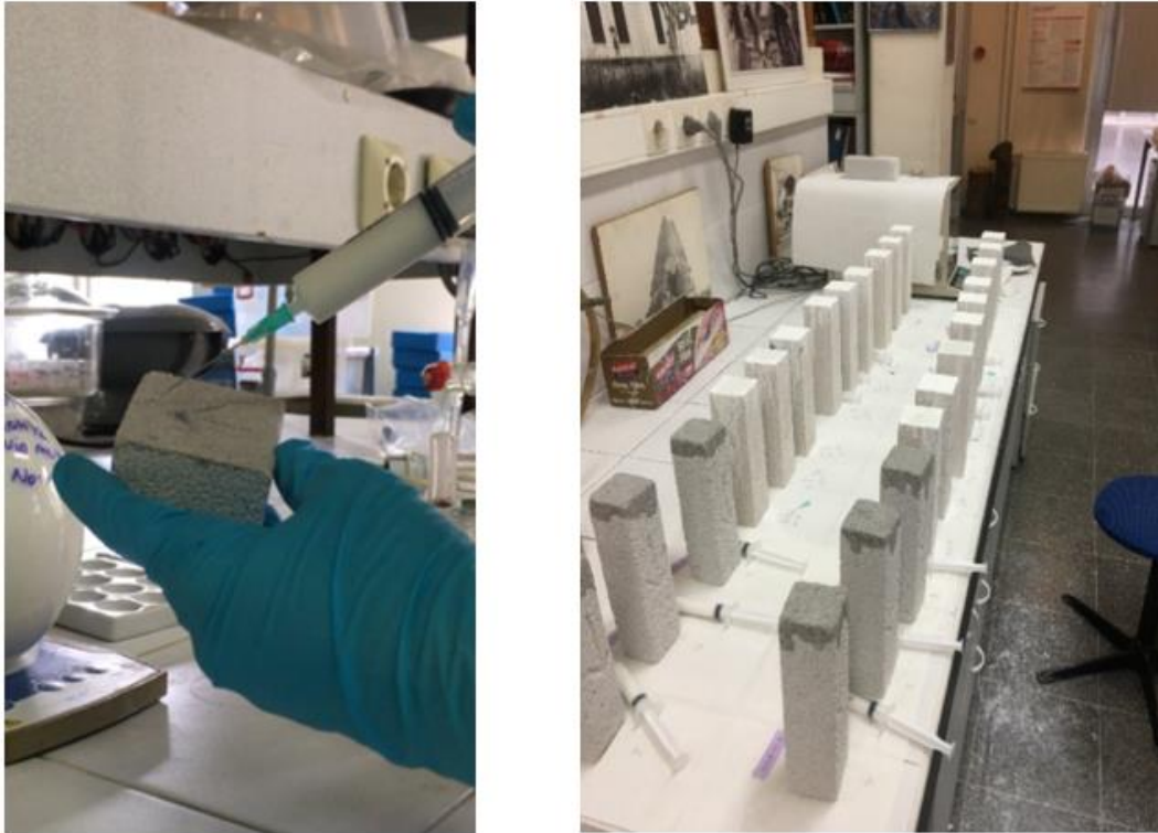
Figure 3.3. Application method of the alcohol-based nano dispersive ( \text{Ca}(\text{OH})_2 ) solution for treatment of AAC samples.
