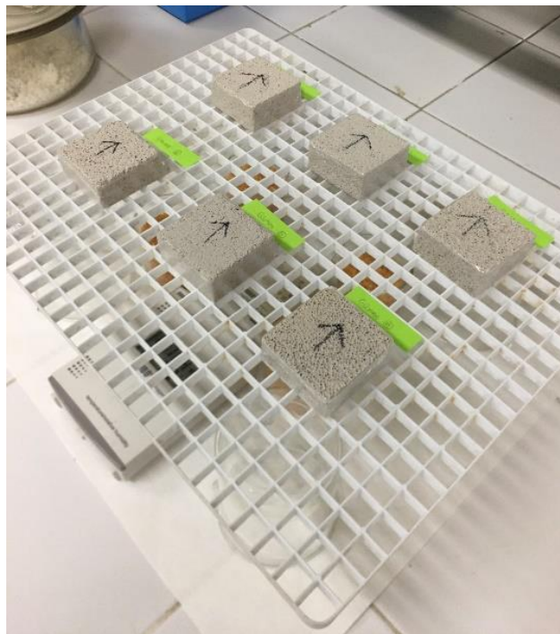
Figure 3.7. AAC samples left for drying at constant conditions of 21±4°C and 30±3% RH.
