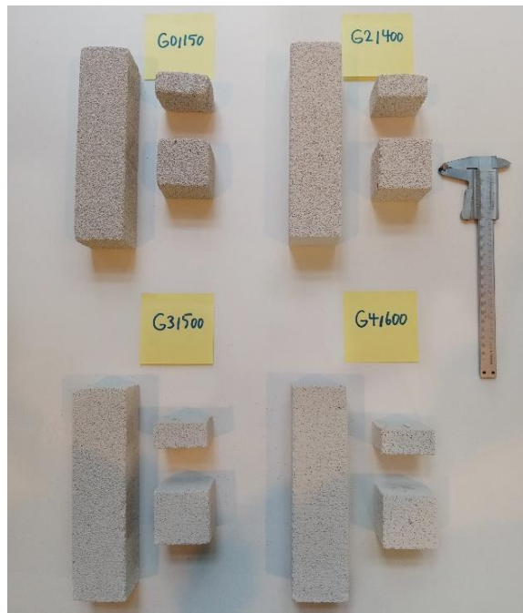
Figure 3.1. AAC samples taken from the local manufacturer used for the sample preparation with dimensions of 5×5×20 cm (left), 5 ×5×2.5 cm (up), 5×5×5 cm (down) for each type (from left side, respectively; G0/150, G2/400, G3/500, and G4/600).
